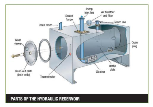
The reservoir plays several important roles. First, it allows any solid contaminants to settle at the bottom of it, ensuing the purity of the system and reducing contamination that could cause failure.
