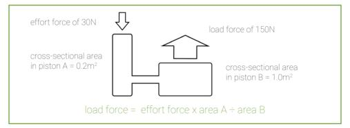
The pressure within this closed system is transmitted equally in all directions, therefore the pressure in piston B is also 150 Pa.
